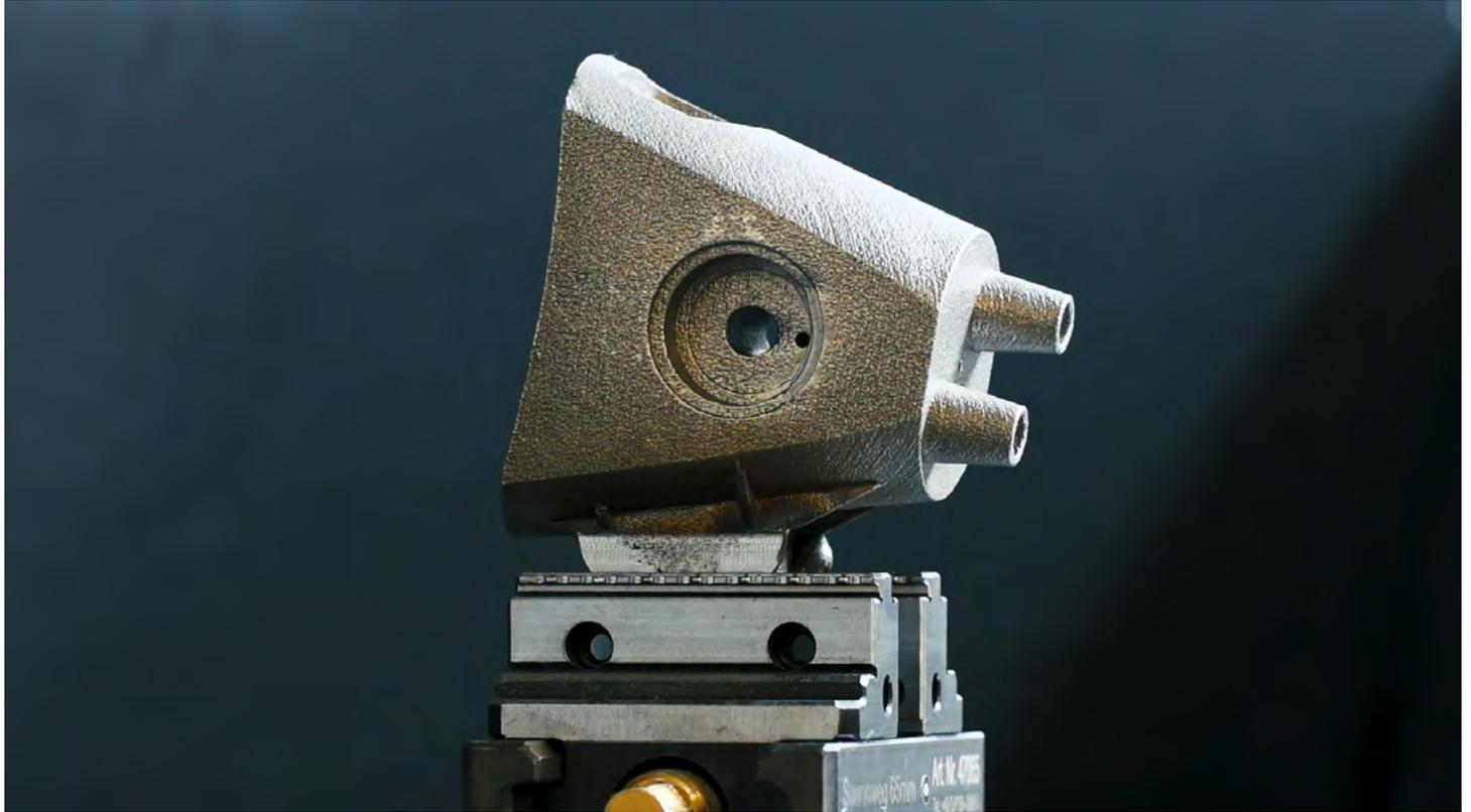
The process is as follows: the scanned data from a clamped printed object is compared with its CAD information, and in this way it is possible to determine the scanned orientation with respect to the clamp, as well as the optimal fit to mill the net shape object with the required tolerance. The CAM NC-code is adjusted accordingly, resulting in the specific NC-code which enables the clamped object to be machined into its net shape.
